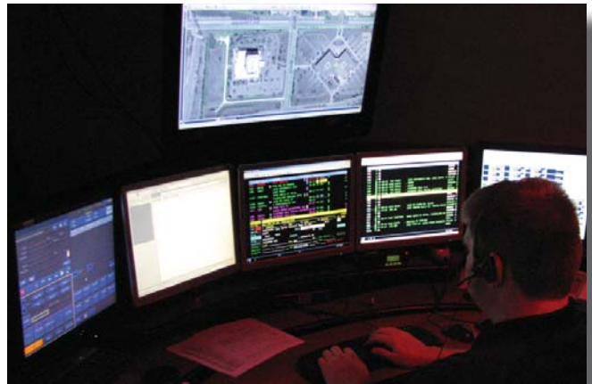
A Public Safety Answering Point features upgraded emergency call-taking equipment that is a component of Iowa's NG911 system.
